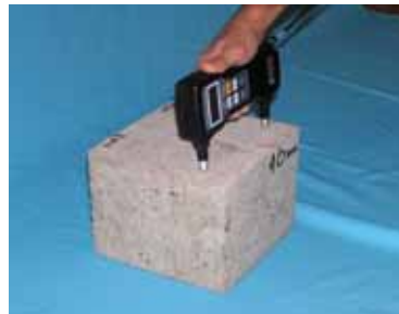
Measure transit time ( t_c ) across crack
