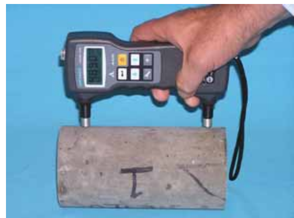
Measure transit time ( t_c ) across crack
