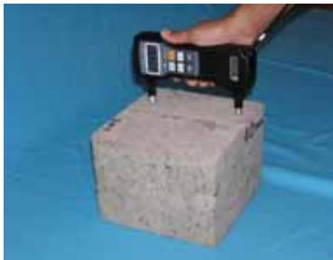
Measure transit time ( t_p ) parallel to crack
