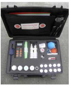
The manual included in the **RCT**-500 kit covers testing for acid and water-soluble chlorides in hardened as well as in fresh concrete. Separately delivered is a binder (RCT-1100) with 15 years of testing experience, including an advanced theory for chloride diffusion modeling.
