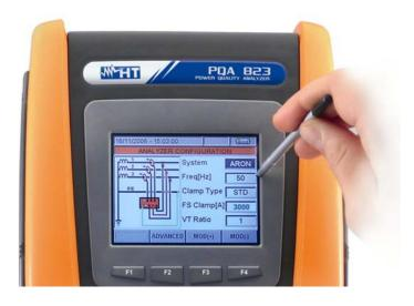
A wide (320x240pxls) graphical color TFT display with "touch screen" to surf the internal functions by using the supplied pointer pen
