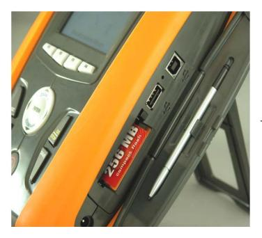
The internal memory (15Mbytes) can be expanded by using the compact flash cards. The instrument has also an USB type A socket to drive USB peripherics like pen drives
