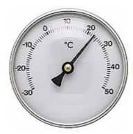
A very useful low cost instrument for measuring the temperature of steel substrates in locations which are structurally difficult to get at, i.e. Bridges, Large Building Frames, Oil rigs etc.
