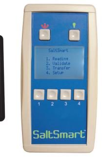
Salt ions are an invisible threat to surface coatings., and they are virtually everywhere and on every surface. There are many kinds of salts, and the ionic compounds formed may be comprised on chlorides, sulfates, nitrates and other chemical compositions. The basic nature of salt is hygroscopic, meaning that when salts are exposed on a substrate they attract moisture that can lead to flash rusting.
