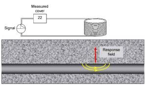
Magnetic field induced by decaying eddy currents in bar
