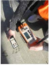
right). The instrument measures the amplitude of the induced current, which depends on the orientation, depth, and size of the bar. The search head is directional and maximum signal is obtained when the bar is aligned with the long axis of the search head. The pulse-induction technique is uniquely stable, is not affected by moisture in concrete or magnetic aggregates, and is immune to temperature variations and electrical interference.
