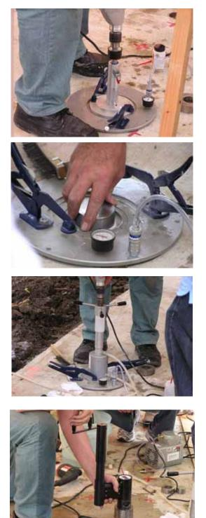
The procedure and special equipment used for the **BOND-TEST** ensure that the disc is loaded in direct tension without bending. Bending may lower results by 20 to 50 %. The discs have sufficient stiffness to avoid distortion during testing. By bonding a clean disc on a planed, dry surface with the GRA adhesive, failure should not occur at the disc/overlay interface. Failure at the disc/overlay interface is an inconclusive test and must be repeated if the bond strength is to be evaluated.
