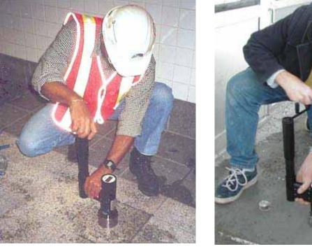
**BOND-TEST** being performed on granite tiles in a subway station
