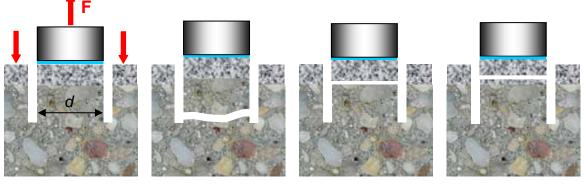
**BOND-TEST** (a) Failure in substrate (b) Bond failure (c) Failure in overlay
