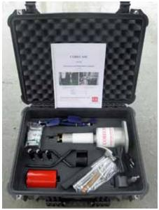
**CORECASE CS-75:** For producing the partial core.
