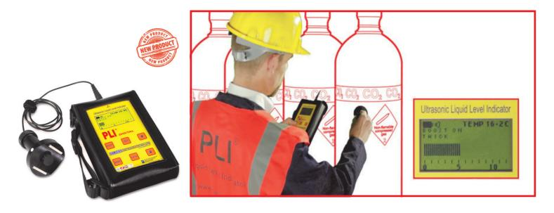
The PLI Digital Portable Liquid Level gauge is designed to offer a simple, accurate, rapid and reliable method of determining the liquid level of high or low pressure CO<sub>2</sub>, Halon, FM200, Propane and any liquefied gas under pressure, without the need to move or weigh the cylinders.
