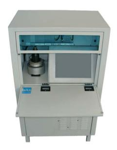
The complete filter skate is inserted manually into the slot before starting the operation. It is strongly advised to insert a "fresh" filter into the slot even for background measurements. Filter-shaped calibration standards (137Cs for the gamma detectors and 239Pu/90Sr for the alpha-beta detector) are required for regular gain and efficiency control.
