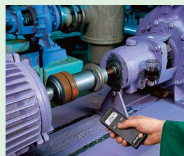
rpm measurement on shafts, rollers etc. using testo 465
